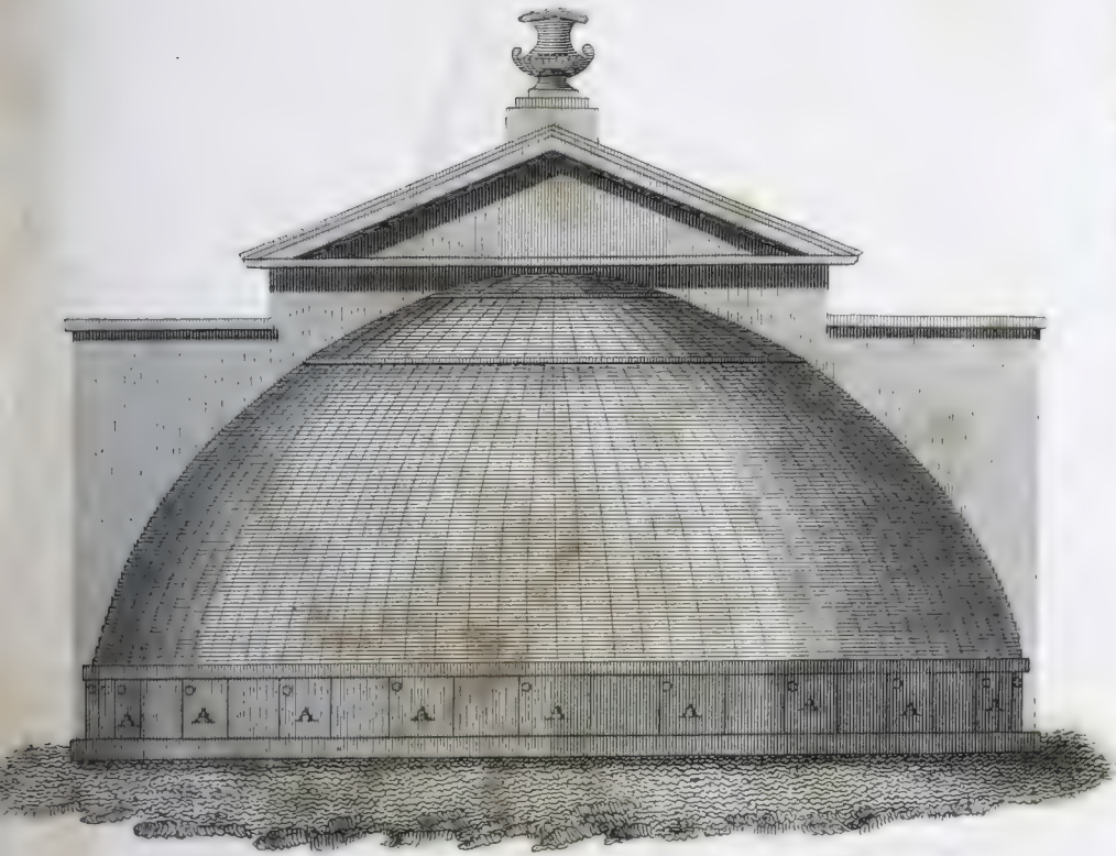
Hot house invented by Sir Geo. Mackenzie Bar t being a Portion of a Sphere. A Segment 31 feet long, 11 high & 13 wide, is recommended as the best size.
